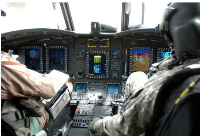
Figure 1 | The Degraded Visual Environment Pilotage System (DVEPS) synthetic vision technology enhances situational awareness and visual cues to pilots. Photo courtesy of Rockwell Collins
