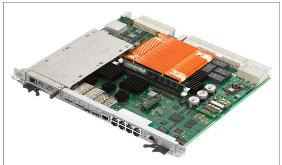
Figure 1 | 40 G ATCA switch blade architecture (Emerson ATCA-F140).
