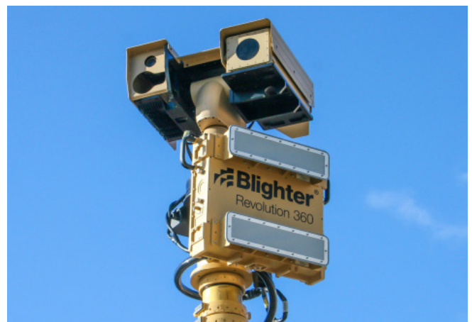
Figure 2 | The Blighter Revolution 360 e-scan radar is capable of detecting figures and vehicles long-range. Photo courtesy of Blighter Surveillance Systems
