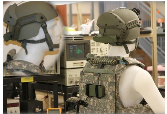
Figure 1 | Prototypes of vest-pocket batteries to power helmet lights and other soldier-worn electric devices have been successfully demonstrated.
